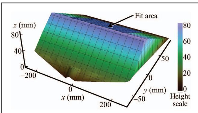
Figure 4. Block used as flat sample for WLS400 test
