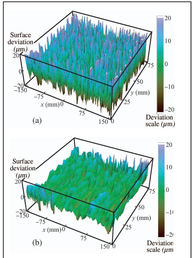
Figure 5. Measurement noise and actual surface deviation, before (a) and after (b) statistical noise reduction
