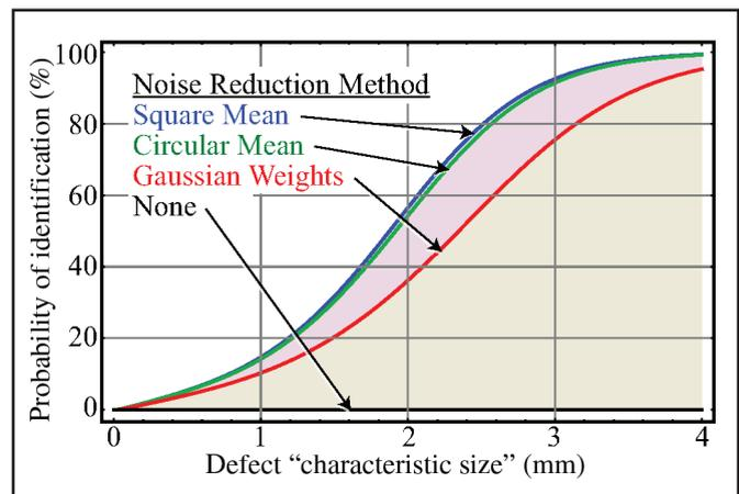
Figure 3. Probability of identifying a  $3\text{-}\mu\text{m}$  feature with no noise reduction (black), Gaussian-weighted noise reduction (red), circular-mean noise reduction (green), and square-mean noise reduction (blue)
