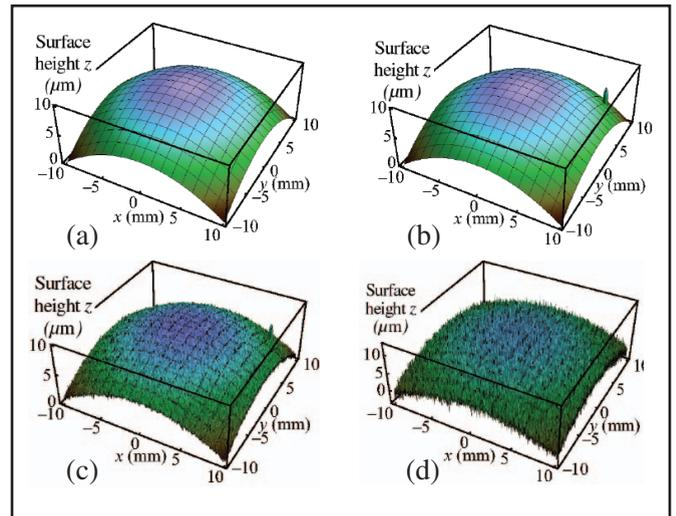
Figure 1. Nominal surface (a) has a defect (b), still visible with low noise (c), but hidden by moderate noise (d)
