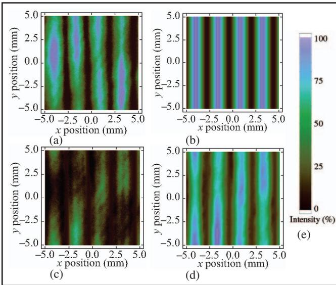
**Figure 8.** Noise reduction in interferometry: the original interferogram (a) was fit to a sinusoid with intensity varying from 0 to 1 (b); the difference between these two is the noise pattern (c); after noise reduction, the interferogram is much clearer (d); all follow the scale (e)
