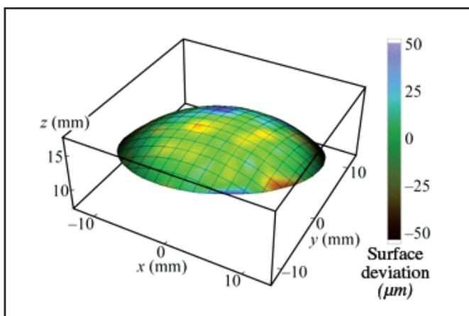
Figure 7. Surface of the sphere with locations measured from its center; surface color shows deviation from nominal (after noise reduction)
