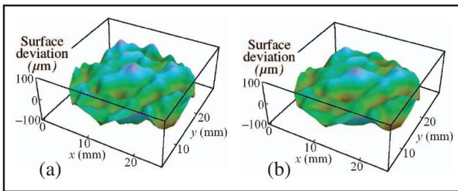
Figure 6. Surface deviation residuals before (a) and after (b) noise reduction
