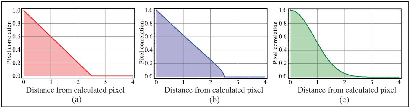
Figure 2. Correlation induced by statistical noise-reduction processes, shown assuming statistical range of 5 pixels for (a) square mean sampling, (b) circular mean sampling, and (c) Gaussian-weighted sampling
