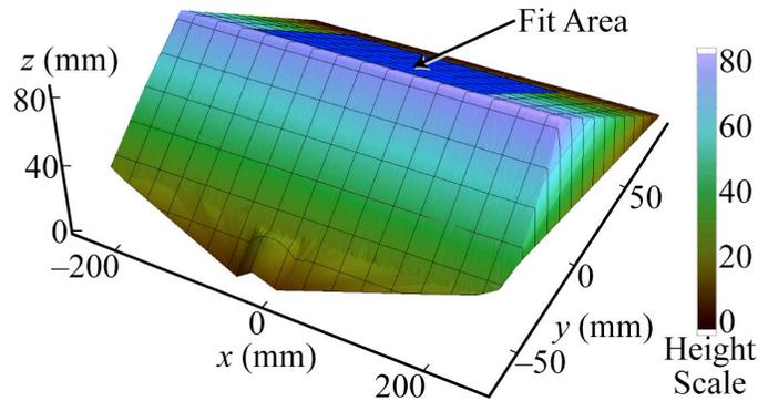
Fig. 4. Block used as flat sample for WLS400 test.
