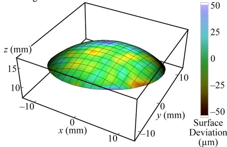
Fig. 7. Surface of the sphere with locations measured from its center. Surface color shows deviation from nominal (after noise reduction).
