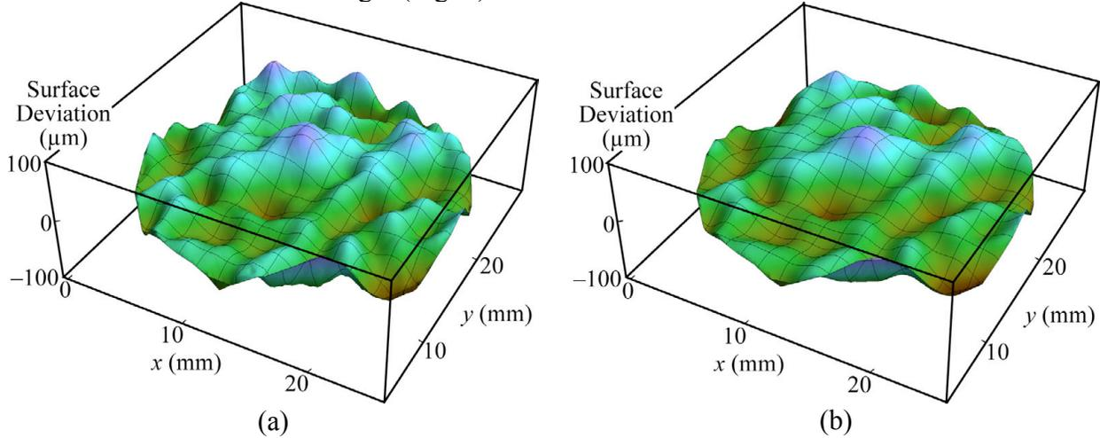
Fig. 6. Surface deviation residuals before (a) and after (b) noise reduction.
