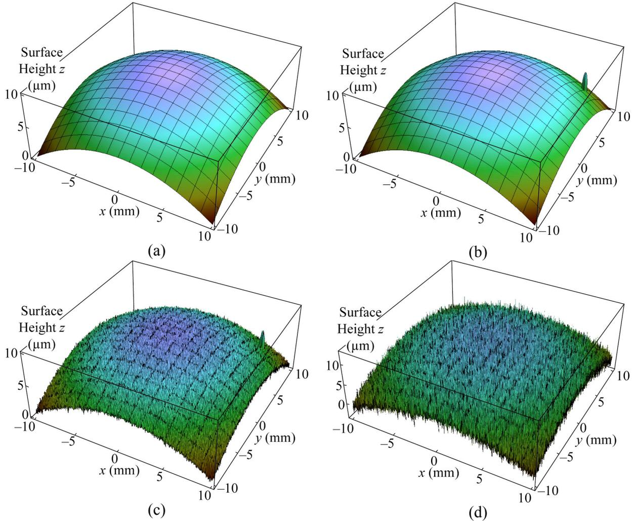
Fig. 1. Nominal surface (a) has a defect (b), still visible with low noise (c) but hidden by moderate noise (d).
