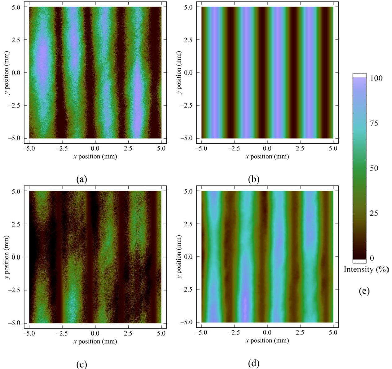
Fig. 8. Noise reduction in interferometry. The original interferogram (a) was fit to a sinusoid with intensity varying from 0 to 1 (b). The difference between these two is the noise pattern (c). After noise reduction, the interferogram is much clearer (d). All follow the scale (e).
