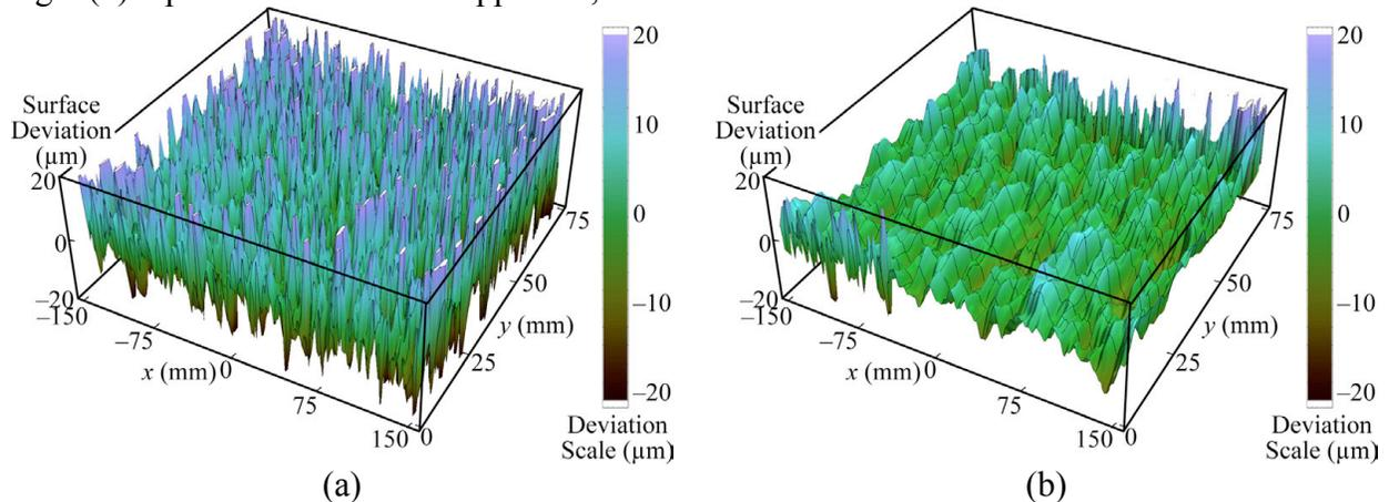
Fig. 5. Measurement noise and actual surface deviation, before (a) and after (b) statistical noise reduction.
