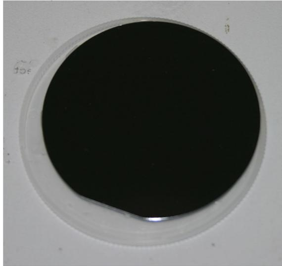
Fig. 2-1. Preliminary photodetector wafer.
